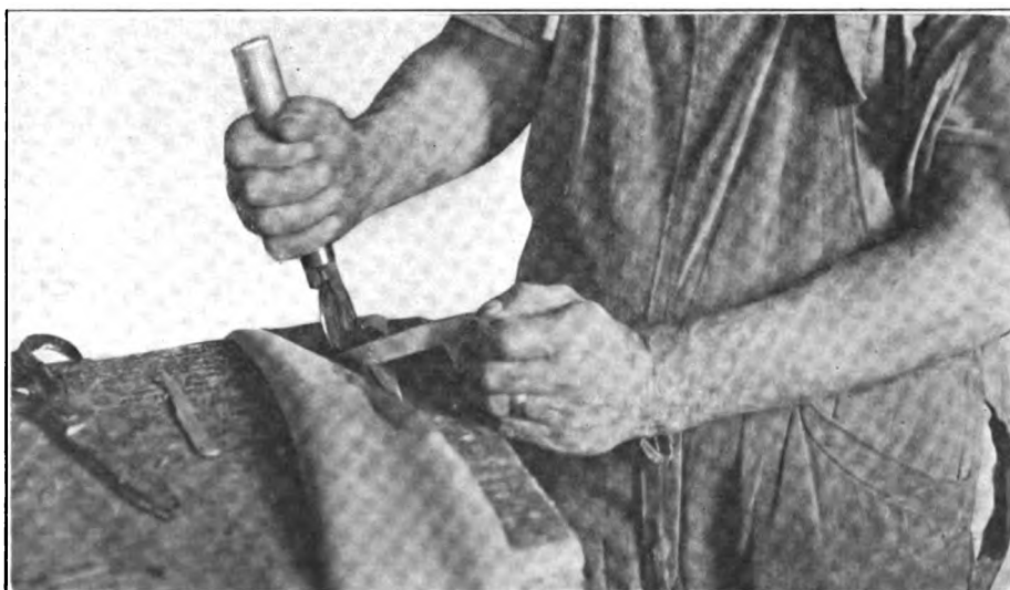
Fig. R—Working in Vulcanizing Gum in a Hole in an Inner Tube Undergoing Repair
